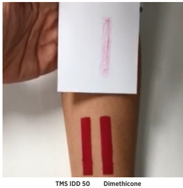
Lip color with 46% TMS IDD 50 exhibited non-transfer whereas lip color with 20% dimethicone exhibited some transfer.
